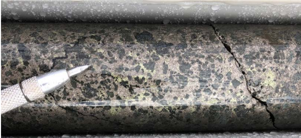
Figure 1. FAVD002 diamond core showing semi-massive sulphides with dominant pyrrhotite and minor chalcopyrite
