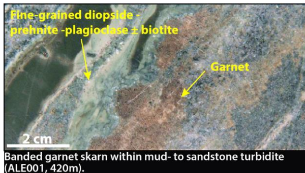
Figure 5. Alteration and host rock examples from the Eaglehawk prospect (ALE001). Core photos and interpretations are re-produced from open file and internal company reports 5,6,7,8 .
