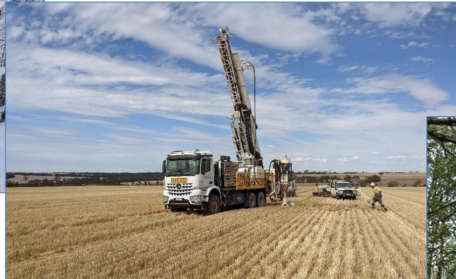
Deeper aircore/RC drilling in WA's wheatbelt
